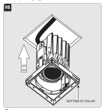
Push the module into the ceiling cut out until the bottom of the collar is flush with or slightly above the bottom of the ceiling.
