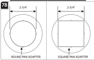
For round trims, mark the location of the 2-3/4" diameter circle on drywall. Use the inside edge of the housing pan adapter as a guide to cut the hole.
