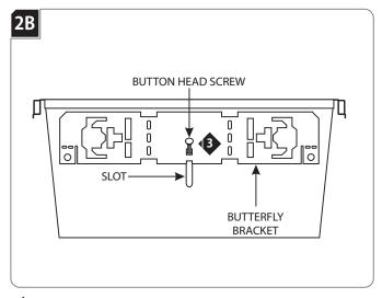
Place the button head screw through the square cut out of the butterfly bracket into the housing slot.
