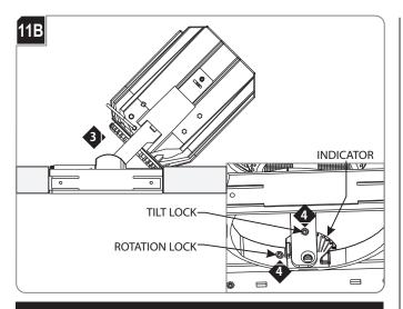
**NOTE:** Module can rotate 361° and tilt to 45° For proper wall wash positioning, tilt until 15° angle is reached.
