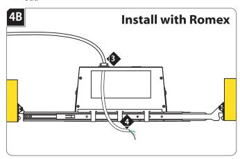
**NOTE:** When using Conduit this step is not necessary, skip ahead to **4C**.
